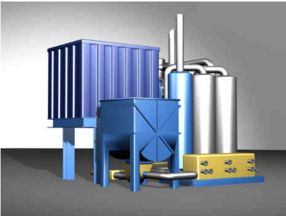
Figure 8 As Figure 5 and 6, but a view that shows the feed hopper with the feed pump underneath.
