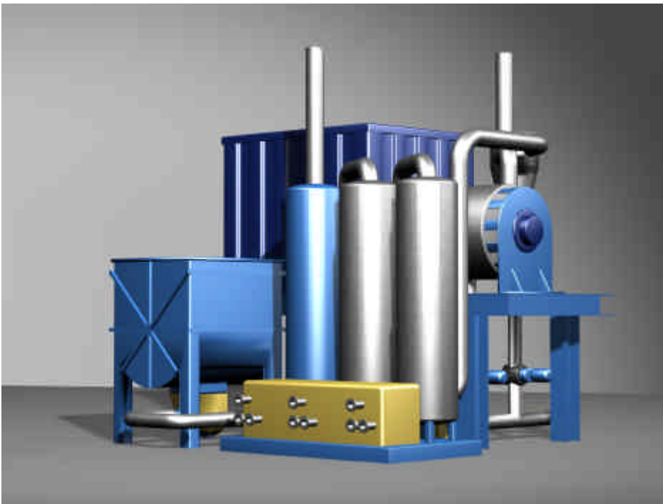
Figure 7 As Figure 5, but a different view. The space required for pumps and valves etc. on the condenser package is shown as a rectangular box for simplicity. The flanges indicate the required pipe connections for coolers and discharge of effluents.
