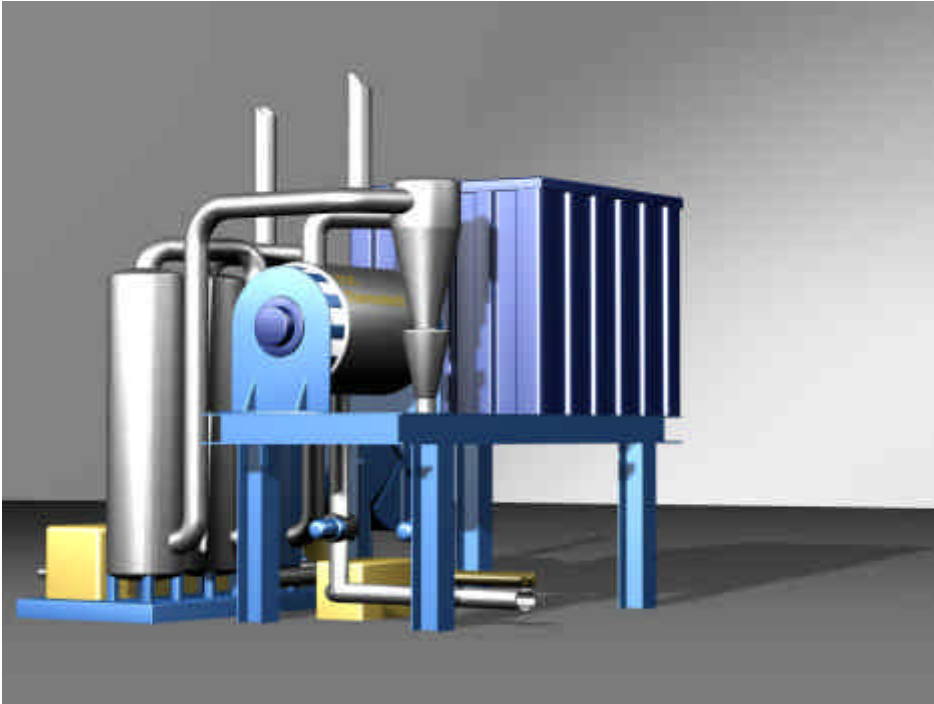
Figure 6 A possible layout for a TCC-450 unit. Footprint 5500×5000×4500
